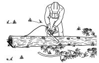
Figure 14 - Bucking Log With Entire Length On Ground
